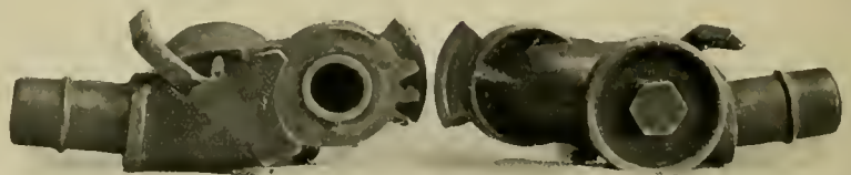
VIEW SHOWING RADLEY'S AUTOMATIC OPENING ANGLE COCK AND HOSE COUPLING UNCOUPLED.
